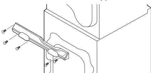
**3** Push open the caps at the left and right sides of the control panel on the front of the appliance. Loosen the screws under the caps.
