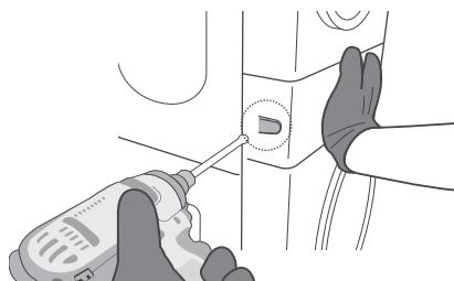
**4** Pull the control panel forward to remove it.
